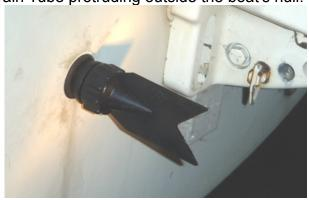
4. When boat is underway, leave Stopper open. For wet storage, either replace the Flapper Valve with the Drain Plug cap, or plug the other end by closing the Stopper.
