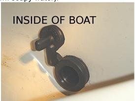
3. Attach Flapper Valve to the notched end of the Drain Tube protruding outside the boat's hull.
